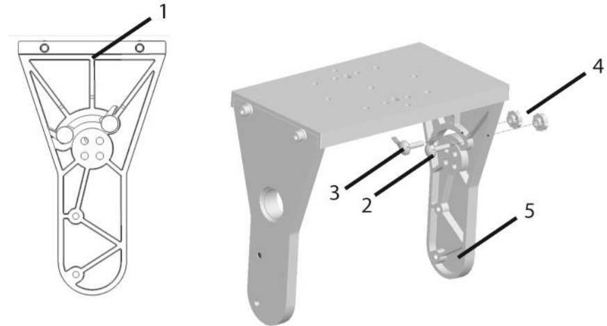
Fig. 8 Over the Top tilt limit adjustment
