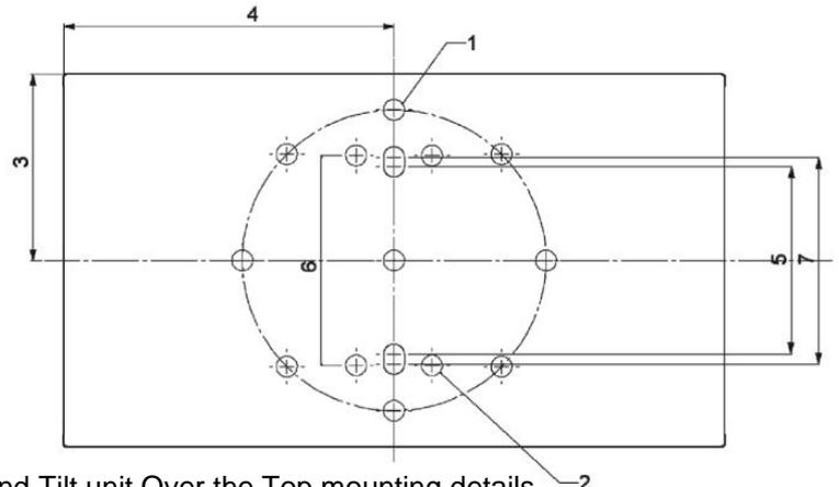
Fig. 3 Pan and Tilt unit Over the Top mounting details
